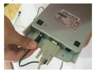
6. Connect the other end of the data cable to the print option plug on the Weishi machine
